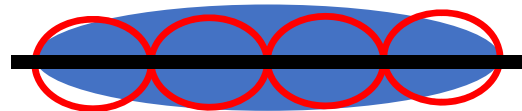
FIGURE 1 Horizontal well to vertical wells [Color figure can be viewed at wileyonlinelibrary.com ]
